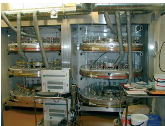
Exposure chambers for rats. The antenna for producing the electromagnetic field is at the centre of each chamber and individual cages for 24 rats are located radially around it
